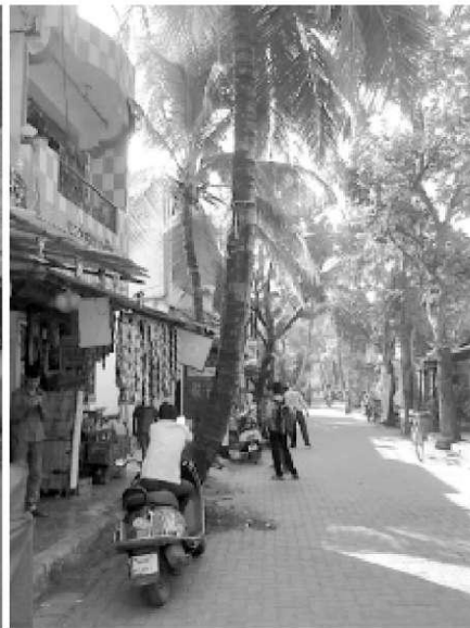
The 9m wide road on to which each courtyard opens. Note that sites-and-services plots abutting the road are allowed to have a shop opening on the street, with the family living space behind the shop. This works well and gives the street a feeling of being busy and active.
